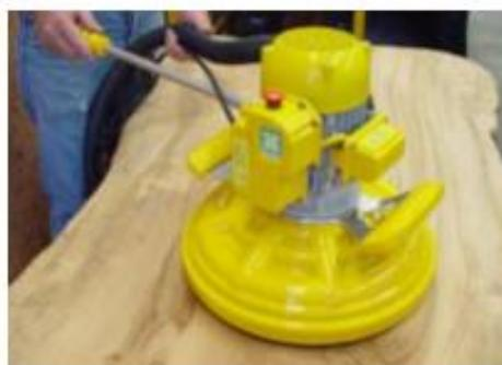
One hand should be positioned on side handle or Quick Release Handle (the vacuum hose and power cord can be cable tied to extension handle, or held away from work surface) whilst the other hand is free to hold edge of fan cowl or turn machine OFF when work has been completed (FIGURE 3)
