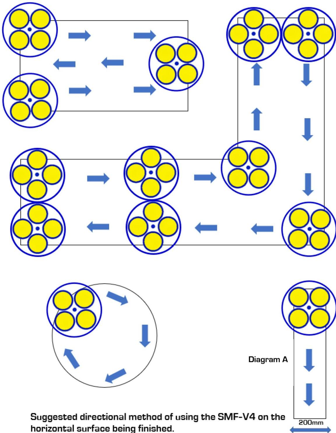
Suggested directional method of using the SMF-V4 on the horizontal surface being finished.
